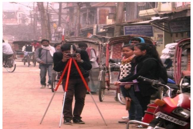
Measurement of Road Alignment by Prismatic Compass Survey in Agartala City Conducted by Dept. of & Disaster Management, Tripura University
