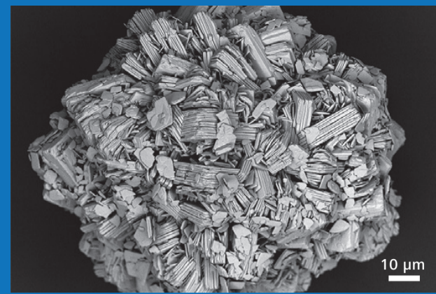
Lanthanum carbonate imaged at 1 kV with InLens Duo BSE. LaCO 3 is a phosphate binder used as a oral therapeutic agent for dialysis patients.
