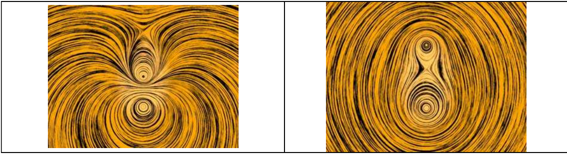
Figure 1.4.6 A flow with two circulation centers with (a) opposite directions of circulation. (b) the same direction of circulation
