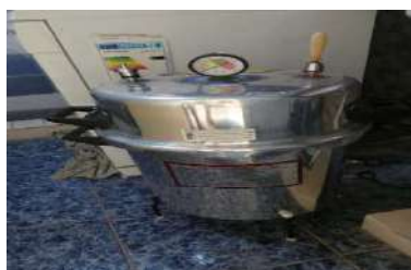
Larger 29L pressure cooker type autoclave
