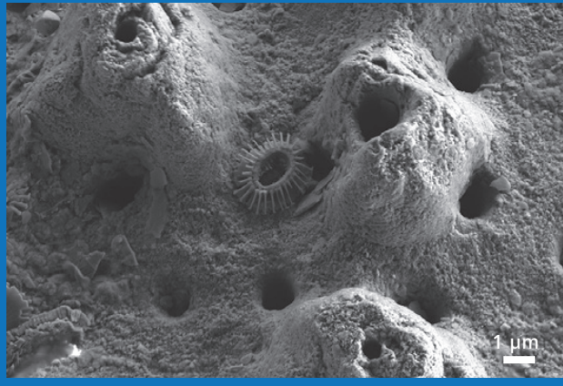
Fine filtered, mixed sediment imaged with the ETSE under high vacuum at 3 kV.
