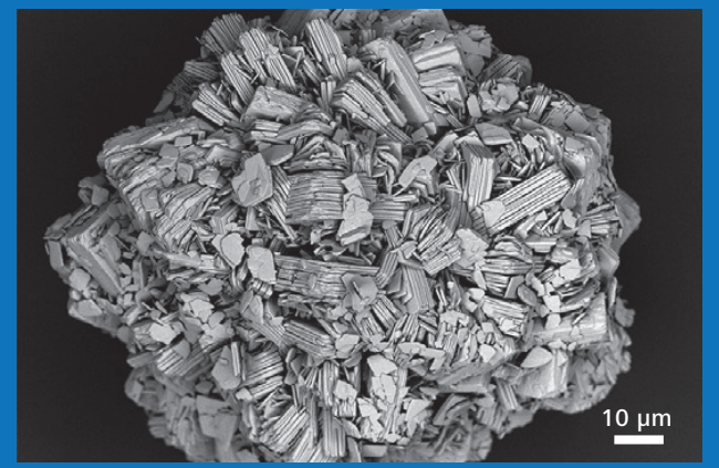
Lanthanum carbonate imaged at 1 kV with InLens Duo BSE. LaCO 3 is a phosphate binder used as a oral therapeutic agent for dialysis patients.
