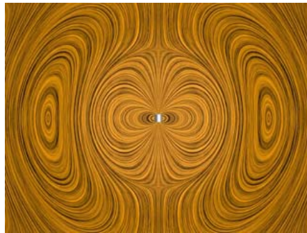
Figure 13.8.6 Radiation from an electric dipole whose dipole moment completely reverses with time.
